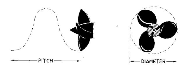
Pitch = 17 Diameter = 14 Pitch and Diameter are the two basic dimensions of a propeller. Example of propeller dimension:  $14 \times 17$
