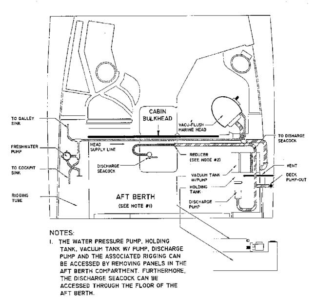
2. THE DISCHARGE HOSE IS REDUCED AND THE MATERIAL IS CHANGED IN THE AFT BERTH COMPARTMENT.
